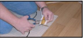
Easybind will fray when cut so to prevent this apply adhesive tape around the rope at the cutting point.
