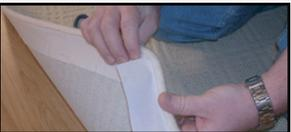
When going around an outside corner cut the binding not the rope and fold underneath, the same applies to an inside corner without the need to fold the binding on the back.
